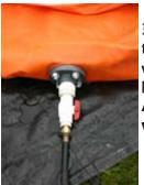
3. Connect hose to tank. Begin filling tank with clean pond water before pond is drained. Avoid hot surface water or muddy water.
